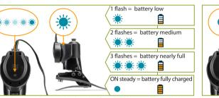
When the IC pod is attached to the foot and being charged, theAfIC pod LED light will pulsate slowly between ON and OFF andopthe charging LED on the foot will indicate charging status ofICthe battery by flashing repeatedly – refer to diagrams.charging LED
