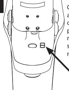
Cover appropriate lines on carrier with permanent black marker to leave spring set number showing.
