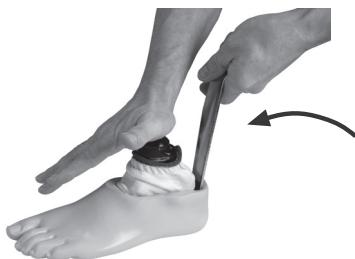
Insert shoe horn behind Heel Spring.
