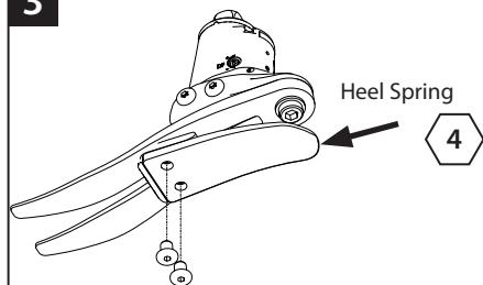
Remove heel spring and screws.
