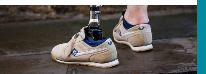
Echelon's biomimetic design follows the same sequence as the human foot: the hydraulics absorb and dampen energy at heel strike and, unlike elastic or fixed ankles that tend to apply unnatural forces, Echelon allows the tibia to stay in a natural position, while the foot self-aligns to the ground. Energy is then transferred through the carbon springs during tibial progression and returned at just the right time at toe-off.
