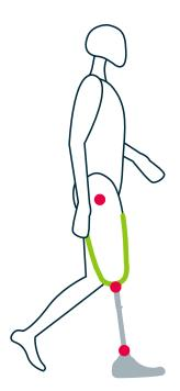
In addition to the ankle, knee and hip, the residuum-socket interface acts as an extra lower limb joint
