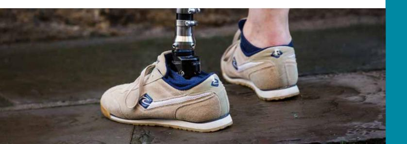
Echelon's biomimetic design follows the same sequence as the human foot: the hydraulics absorb and dampen energy at heel strike and, unlike elastic or fixed ankles that tend to apply unnatural forces, Echelon allows the tibia to stay in a natural position, while the foot self-aligns to the ground. Energy is then transferred through the carbon springs during tibial progression and returned at just the right time at toe-off.
